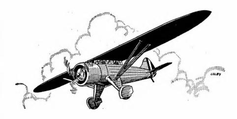
tion with an elliptical plan form. It is made in two sections joined at the center-line. There is a Vee strut on each side of the fuselage. The general structure is a light metal with a fabric covering, but the leading edge is protected with a duralumin sheet. Long tapering-chord ailerons
