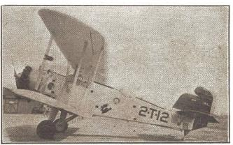
THIS is the Navy's Great Lakes TG-2 dual-purpose plane. It's a threeplacer that can be used either as a torpedo carrier or light bomber. Top speed fully loaded is 127 m.p.h. with the 575-h.p. "Cyclone." She also comes in a scaplane version.
