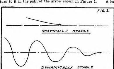
To design a satisfactory flying model, it isn't sufficient that you builders watch your P's and Q's—you've also got to watch your C.G.'s! That's because a flying model must have stability if it's going to be any good at all. So dig into this article, which tells you how to apply these principles at your own model workbench.
