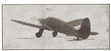
And now we twist 'er around to get a rear-quarter view. Note the wing fillet work, the tail rigging, and the built-in dihedral which gives the craft that anxious-for-the-air smack.
